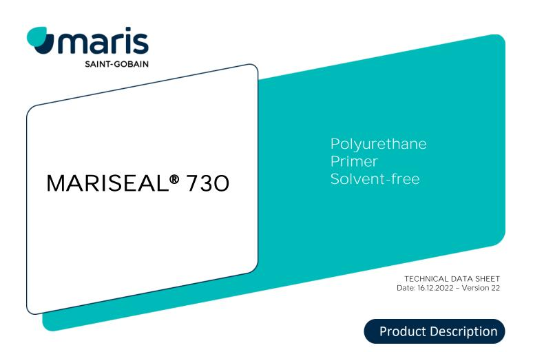
MARISEAL® 730 is a transparent, elastic polyurethane primer. Used as a primer in waterproofing and sealing applications mainly on bitumen/ asphalt felts.
